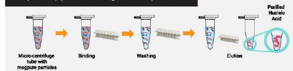
Fig 2: Magnetic bead based purification protocol – The protocol for purifying genomic DNA from various samples using "MAGNXT" purification kits using 4 simple steps- bind, wash, elute, and purify.
